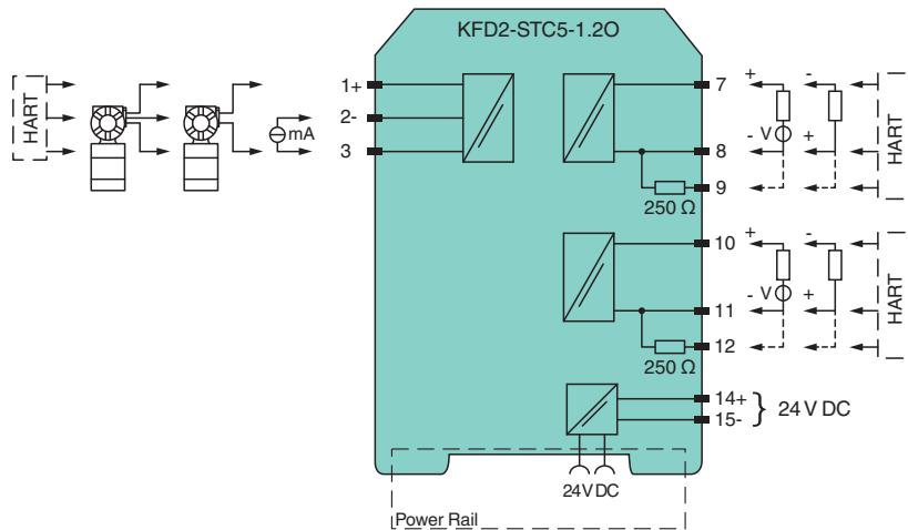
Short circuit unused circuits on the output. Open circuit outputs increase the internal power dissipation by up to 300 mW per channel.
